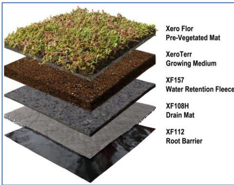
The Xero Flor system is an extensive green roof assembly with lightweight, pre-vegetated mats, delivered with well-developed, mature plants. They roll out like sod for ease of installation. The system is based on a time-tested design originally developed in Germany. In Xero Flor mats, the plants and a layer of engineered growing medium are grown together on a durable geosynthetic textile carrier. All system components for installations in the United States are 100 percent American-made.
